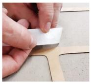
Apply the enclosed adhesive strips onto the backs of the stencils to help keep them in place during coating application. Use sparingly (6 - 10 strips per stencil) or as many as you feel you need.
